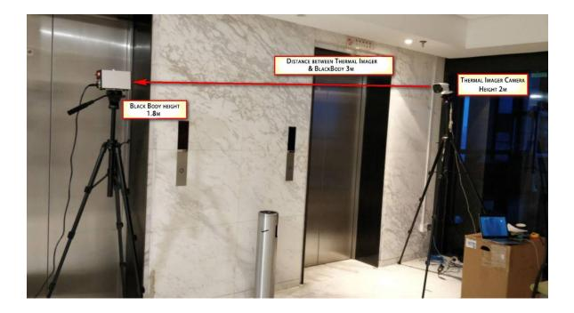
The Thermal Imager Camera device should be position in alignment with the BlackBody Thermal Screen facing the camera device while the Thermal Imager camera to position facing the passageway to avoid view or passage obstruction.
