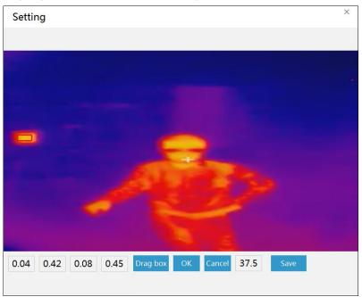
BlackBody non-screening option: For better temperature screening with BlackBody, select BlackBody correction blue icon on top right corner of software, click on "Drag box" and select the BlackBody on the Thermal Imaging window and save settings. This will enable the Thermal Imager Temperature camera to ignore the temperature from the BlackBody for better temperature screening measurement.
